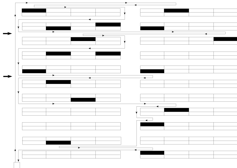
Figure 5. Orderpicking route in the current method with full aisle traveling (lefthand block) and return (righthand block).
